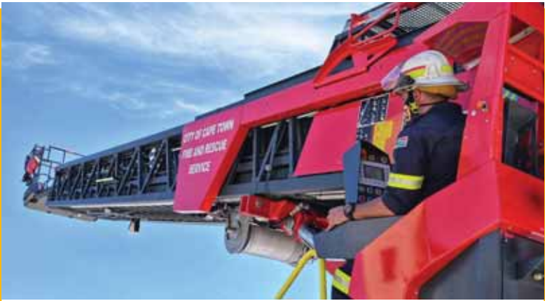
"High" there: The new 56 m turntable ladders can access a 22-storey building.
